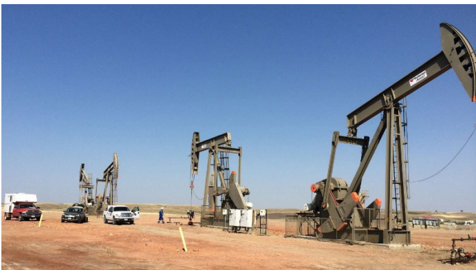
Pumpjacks at oil wells in the Bakken Formation, North Dakota. In these modern oil wells, the derricks used to drill the wells have been removed. Photo by USGS (public domain) .
